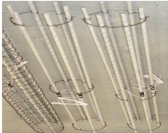
Figure 4: Typical steel and glass FRP cages
