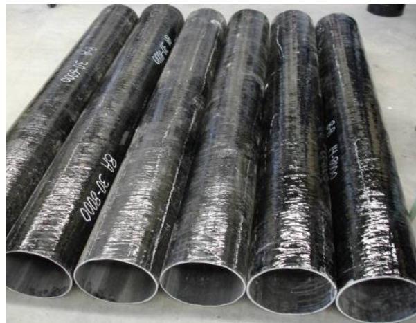
Figure 3: Green FRP tubes for beam specimens
