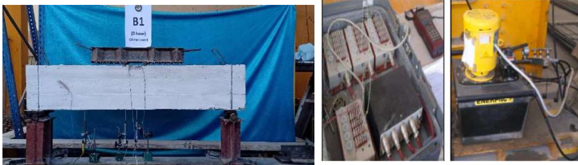
Fig. 6. Experimental Test Setup, Load Cell, and Data Logger and Reader.
