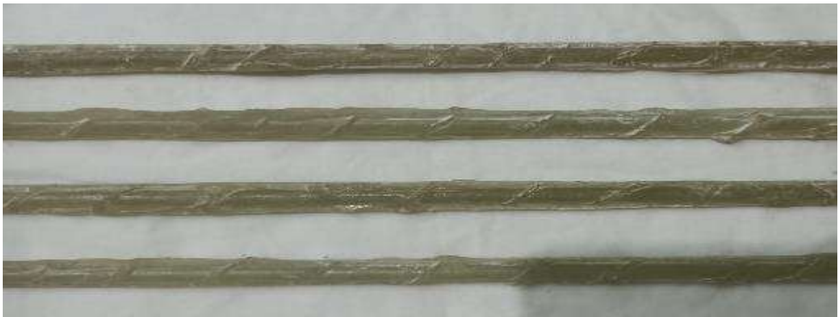
Fif (3): Surface characteristics GFRP bars.
